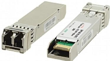
OSP-MM1 is a fiber optic transceiver for 850nm multimode signals. This standard pluggable SFP+ optical module has two LC connectors for reception and transmission of signals over two strands of multimode optical fiber
